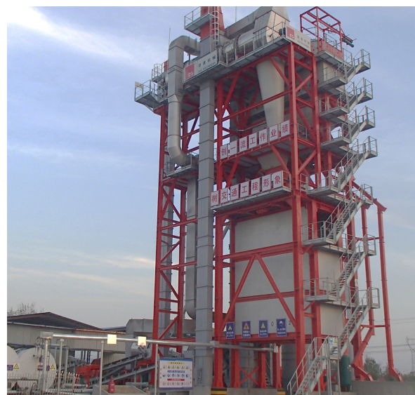
D&G's monoblock recycling asphalt mixing plant
