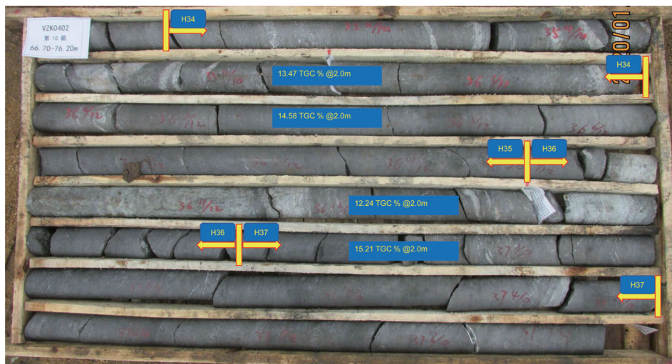
Figure 4–4: Graphitic schist intersected by drillhole VZK0402
